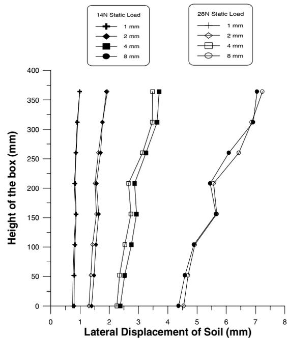
**Figure 3. Lateral soil displacement with height of the box for rigid pile wall**
