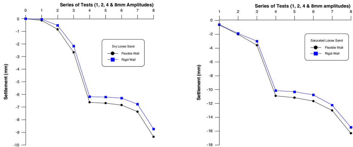
**Figure 9. Variation of settlement with series of tests for flexible and rigid pile walls in loose dry and saturated state**
