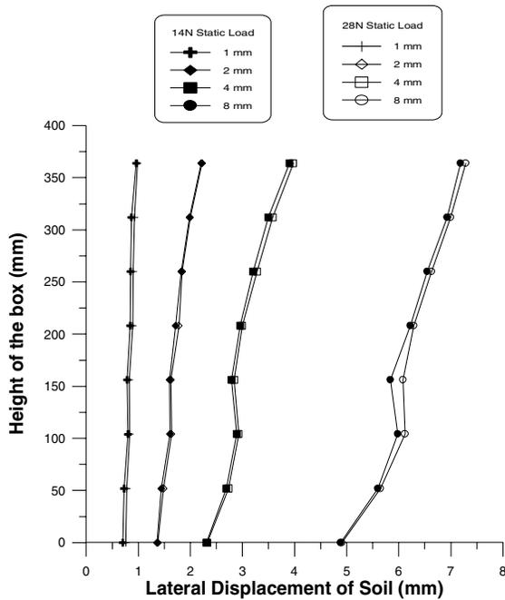
**Figure 6. Lateral soil displacement with height of the box for flexible pile wall**
