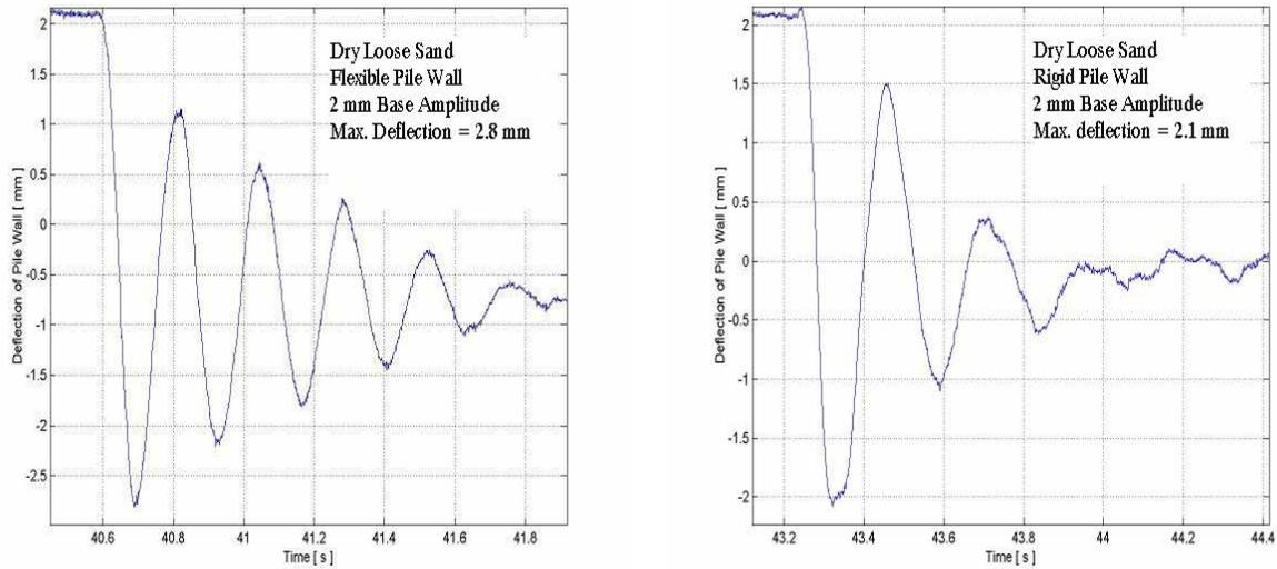
**Figure 4. Variation of deflection at top of the flexible and rigid pile walls with time in dry loose sand with 2 mm base amplitude**
