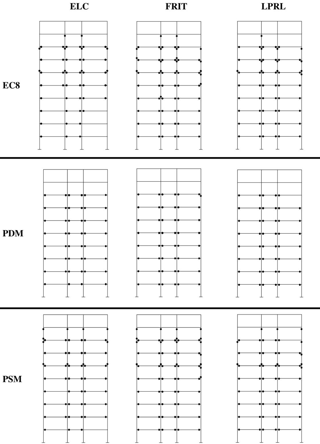
**Figure 8. Plastic hinge distribution in 10-story frames designed to EC8 and Proposed Dynamic and Static Methods (PDM, PSM) for the 3 most critical earthquakes at collapse-prevention level.**
