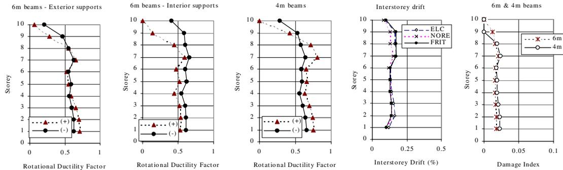
**Figure 3. Maximum response under 3 immediate-occupancy (serviceability) level earthquakes for partial inelastic modeling of 10-story frame, (Drift values are shown for each earthquake).**
