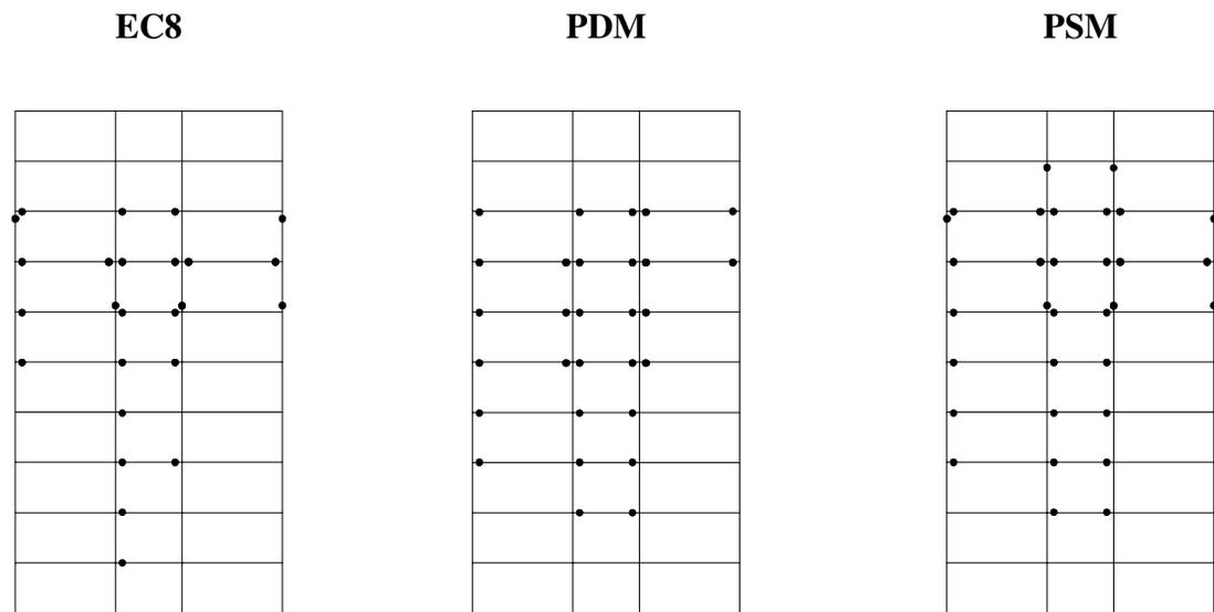
**Figure 7. Plastic Hinge Distribution in 10-story frames designed to EC8 and Proposed Dynamic and Static Methods (PDM, PSM) for the most critical earthquake (FRIT) at life-safety level (0.25g).**
