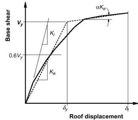
**Figure 1. Calculation of effective stiffness  $K_e$  [23]**
