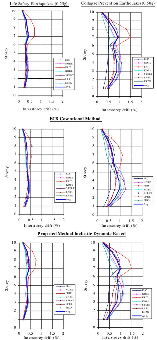
**Figure 5. Interstory drift ratio for 10-story frames designed based on conventional and proposed methods under seven life-safety and collapse-prevention earthquakes**
