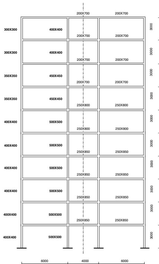
Figure 2, Initial geometry of 10-story frame structure (units: mm)
