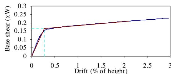
**Figure 4. Base shear vs. global drift for partial inelastic model of 10-story frame**
