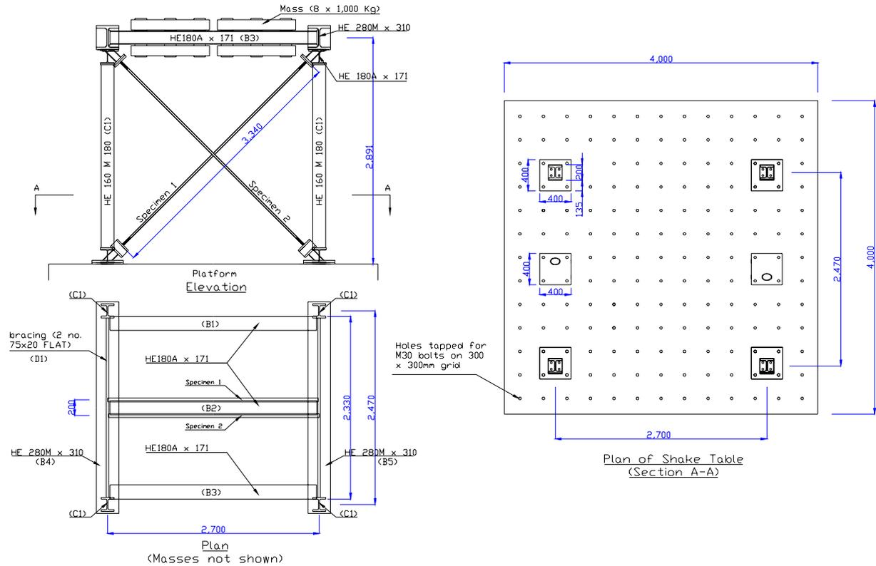
**Figure 1 Experimental arrangement for shake-table tests**
