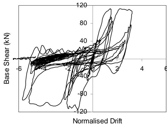
**Figure 6 – Base shear response of H40A**
