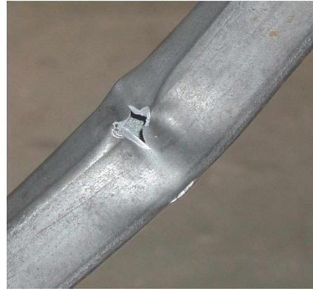
**Figure 7 – Local buckling and partial fracture**
