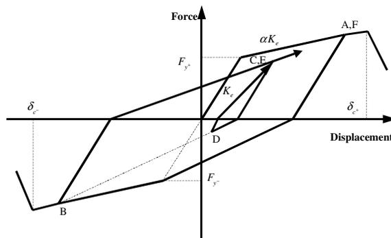
Figure (2) Modified-Clough Model
