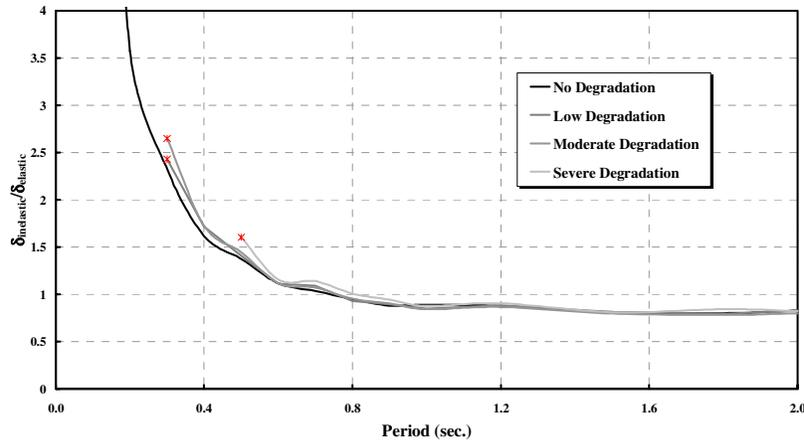
**Figure (9) Displacement Estimates for Pinching Model – R=8**
