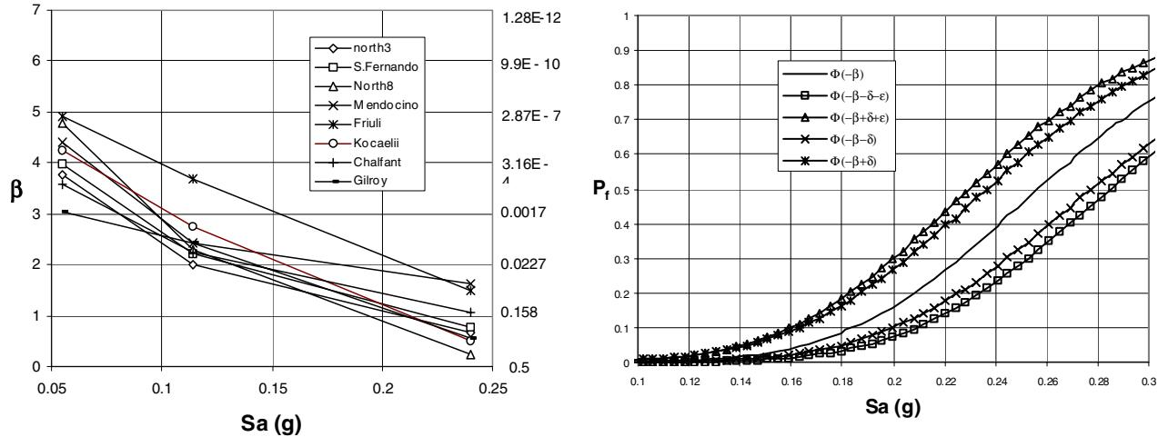
Fig. 5 Olmeta viaduct, pier n. 2: (left) Reliability index  $\beta$  for different accelerograms vs. the spectral acceleration; (right) fragility curve and sensitivity of error model and variability of response.
