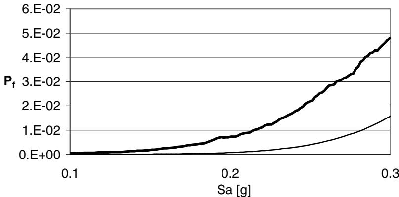
Fig. 6 Cadramazzo viaduct: fragility of the bridge (thick line) and probability of failure at the central point of experiment design (thin line)
