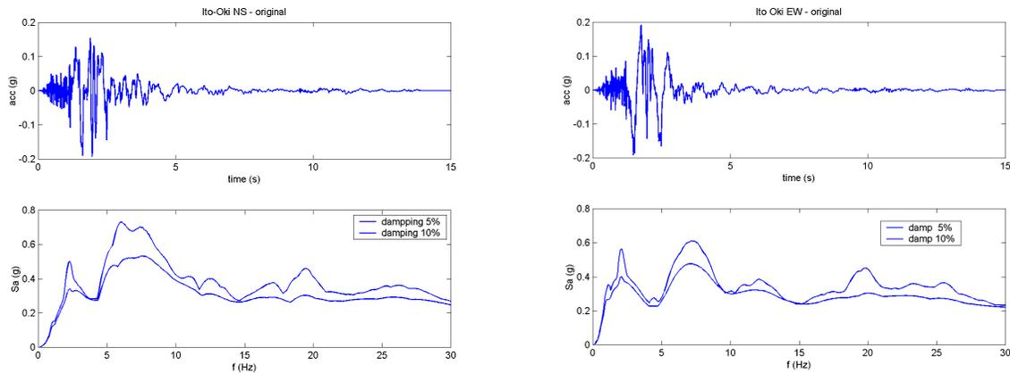
**Figure 1. Time histories and response spectra of horizontal components of Ito-Oki 1989 earthquake**
