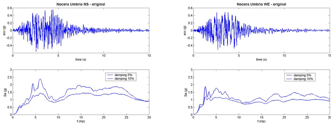
**Figure 2. Time histories and response spectra of horizontal components of Umbria 1997 earthquake**
