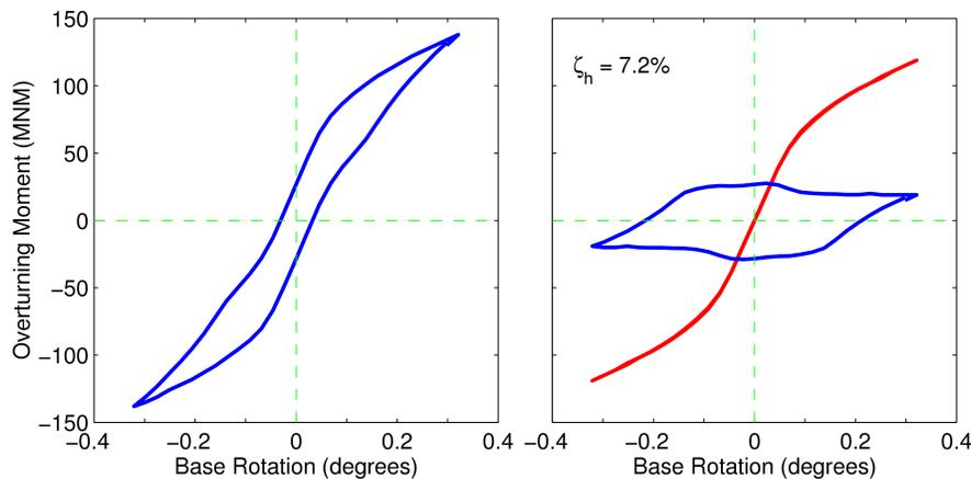
**Figure 2: Overturning moment-rotation relation for partially uplifted base. The skeleton stiffness and hysteresis loop are shown on the right side.**
