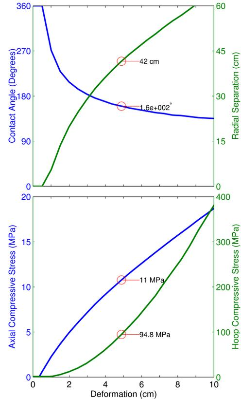
**Figure 4. Contact angle and radial separation (top). Axial and hoop compressive stresses in tank wall (bottom).**
