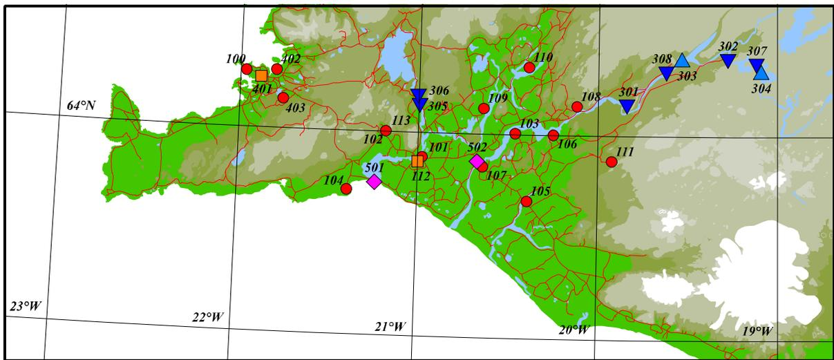
Figure 2: The Icelandic Strong-motion Network. The following notation is used: ● ground response stations, ▼ hydropower stations, ▲ earth-fill dams, ◆ bridges and ■ office buildings.
