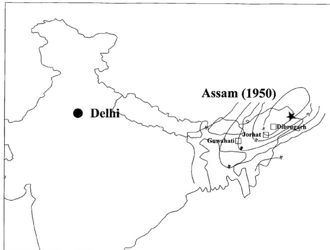
Figure 4 Isoseismal map of the Assam earthquake of August 15, 1950 (Tandon [16]).
