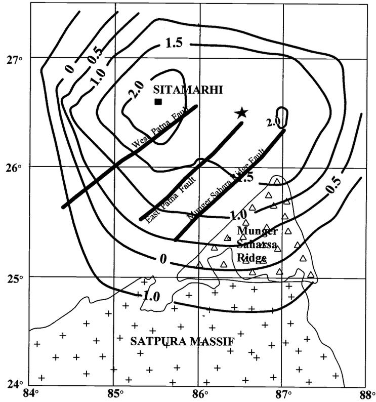
Figure 9a Residual intensities of the Bihar Nepal earthquake along with the geological structures faults and the slum belt.
