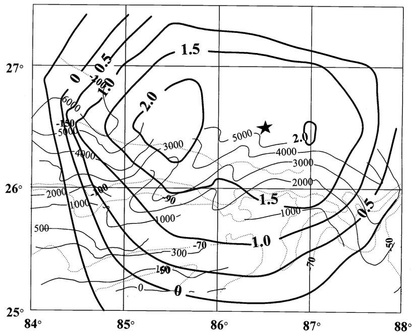
Figure 9b Residual intensities of the Bihar Nepal earthquake along with the Bouguer gravity anomalies and the basement depth (for legend refer figure 8b).
