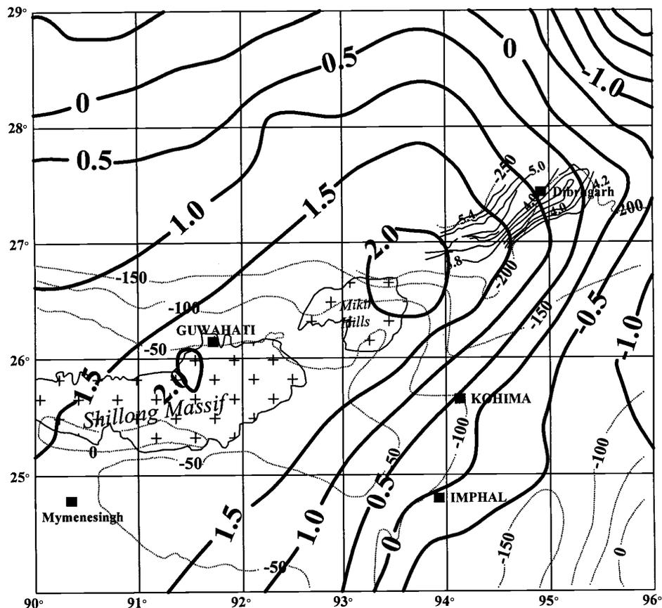
Figure 10 Residual intensities of the Assam earthquake along with the Bouguer gravity anomalies and the basement depth (for legend refer figure 8b).
