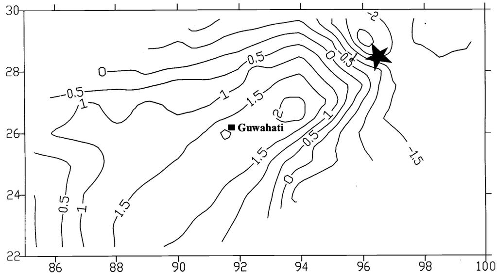
Figure 7 Residual intensity map for the Assam earthquake.
