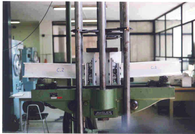
Figure 8. Photograph of the test assembly of the second HLT series, HLT2.
