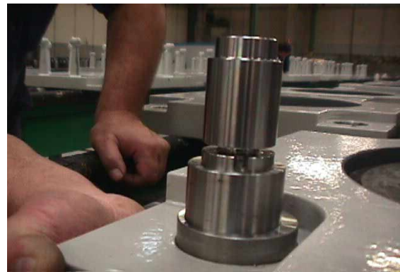
Figure 5. Installation of a sacrificial element in an isolator.
