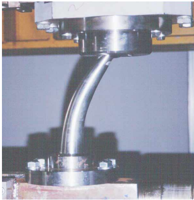
Figure 7. A single tapered pin dissipating element during tests at FIP Industriale laboratory
