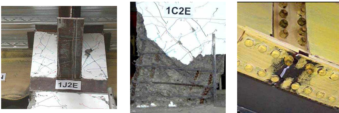
Figure 15 Condition of beam-column joint, RC column base, and bolted beam splice at end of static pushover to 10% interstory drift
