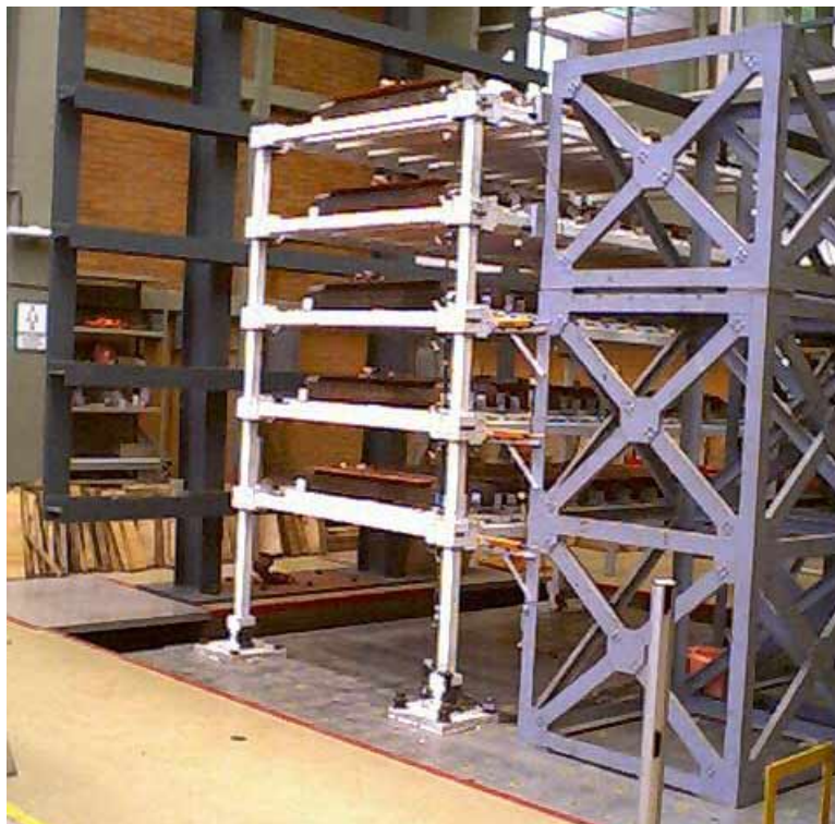
Figure 5. Building on the shaking table
