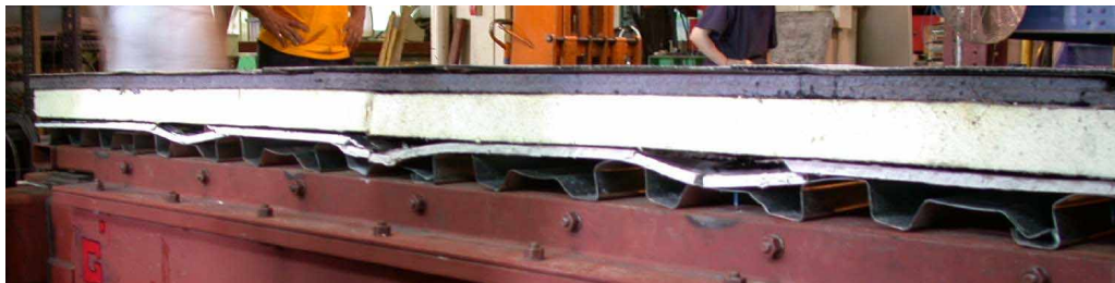
Figure 10 : Warping deformation of steel deck restrained by non-structural components (Test 45)
