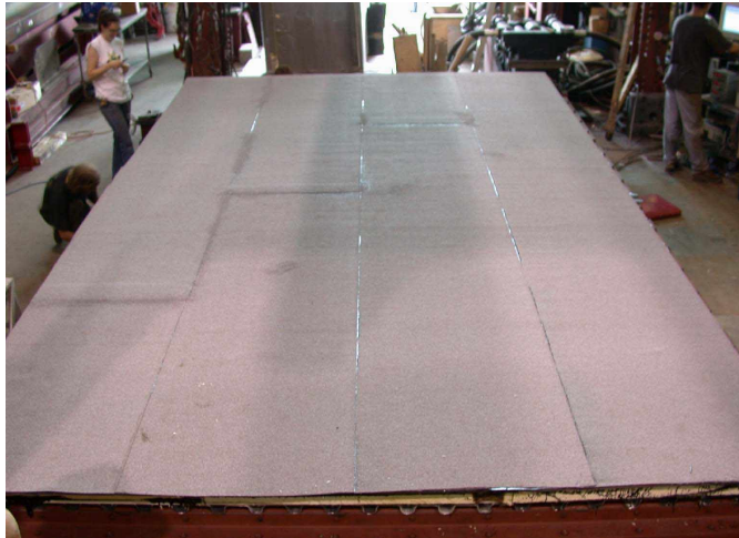
Figure 5 : View of diaphragm specimen with roofing material (Test 45)
