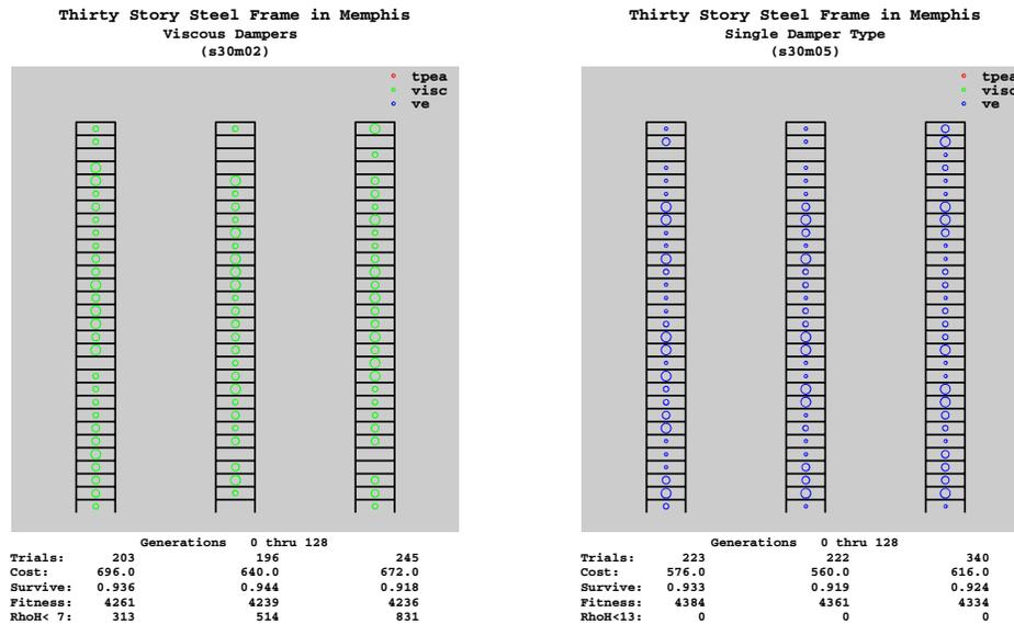
Figure 7: Thirty Story Steel Frame in Memphis, a) Viscous only, b) Single damper type
