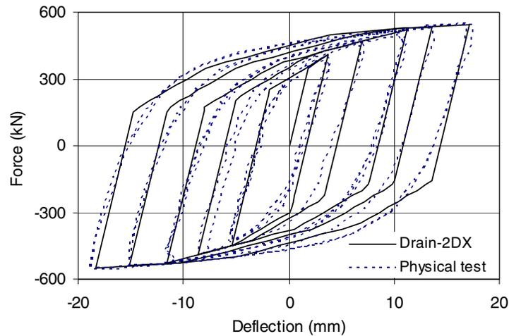
**Figure 3. Comparison of response of Drain-2DX knee element model with cyclic test data**
