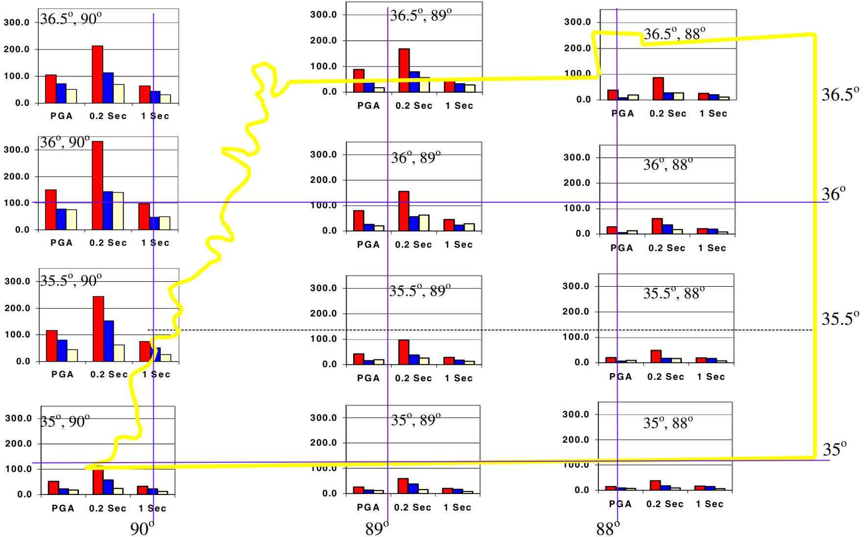
Figure 1. Comparison of PGA, 0.2-Second Spectral, and 1.0-Second Spectral Acceleration Coefficients from Three Different Studies.
