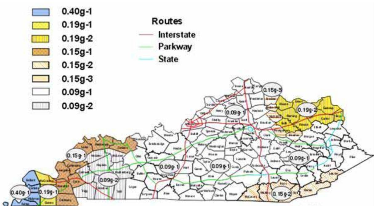
**Figure 1 Seismic Acceleration Map of the 250-year Earthquake Event for the Commonwealth of Kentucky**
