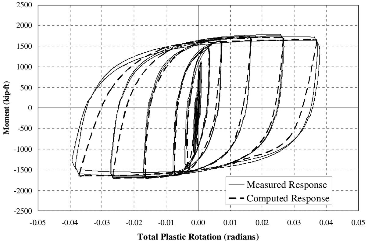
**Fig. 10: Comparison between measured moment versus total plastic rotation for the RBS1 (W14x283 column) specimen.**
