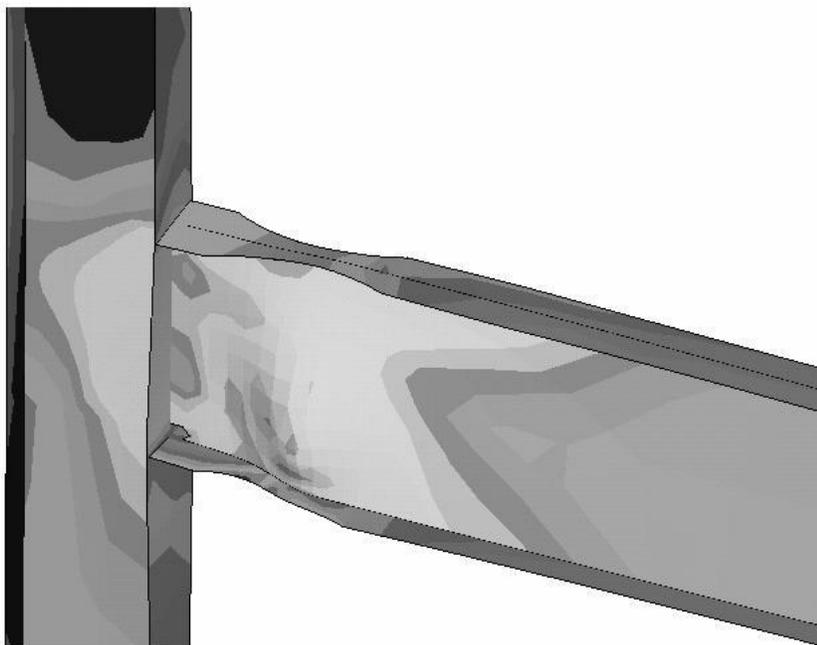
**Fig. 15: Oblique deformed view of the von Mises stress distribution in the RBS3 (W18x211 column) specimen at 0.05 radians.**
