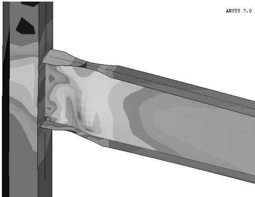
**Fig. 14: Oblique deformed view of the von Mises stress distribution in the RBS1 (W14x283 column) specimen at 0.05 radians.**
