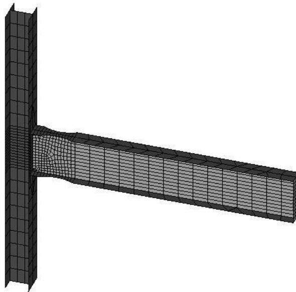
**Fig. 8: Oblique view of the RBS1 (W14x283 column) finite element model.**
