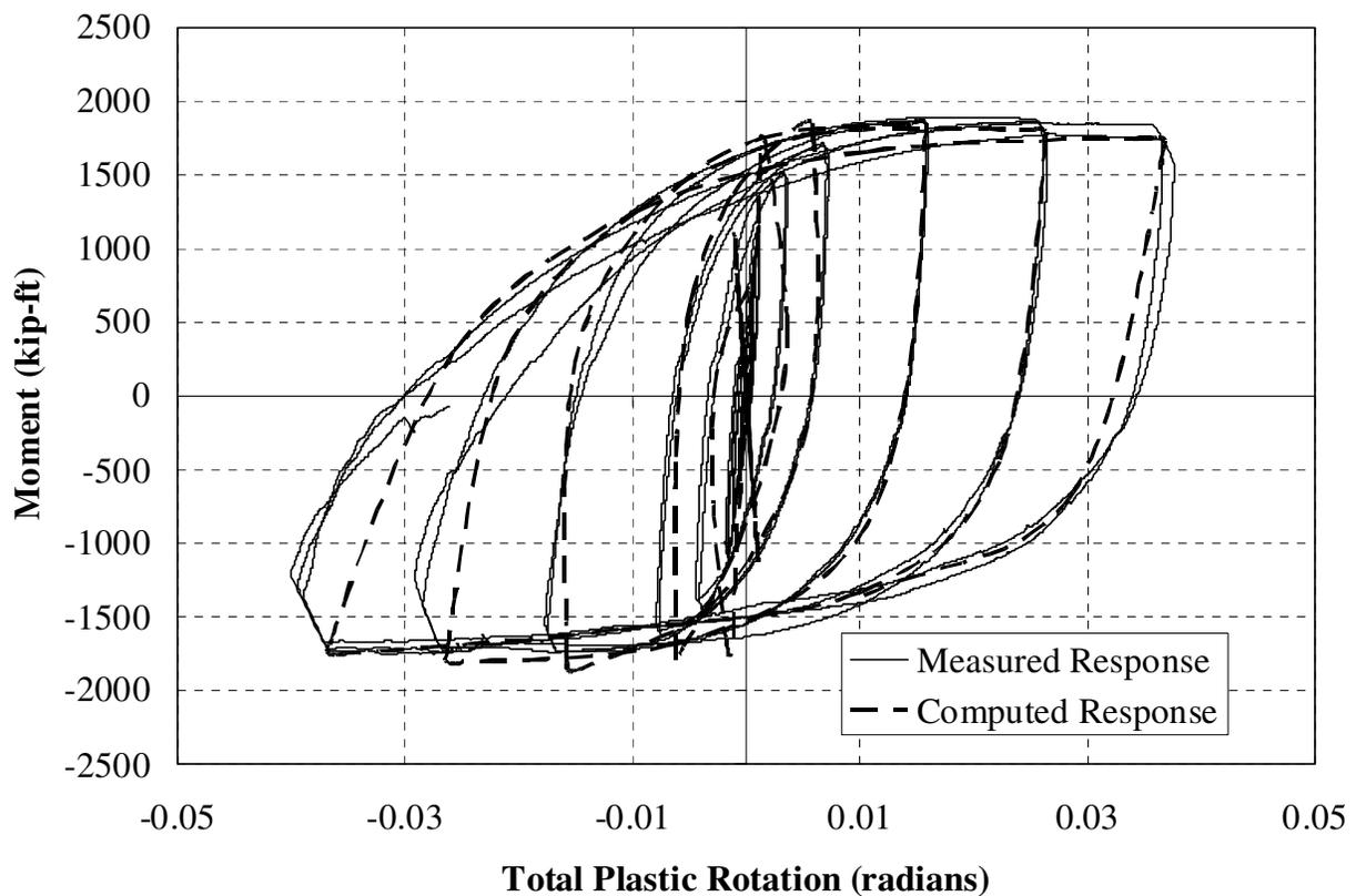
**Fig. 11: Comparison between measured moment versus total plastic rotation for the RBS3 (W18x211 column) specimen.**
