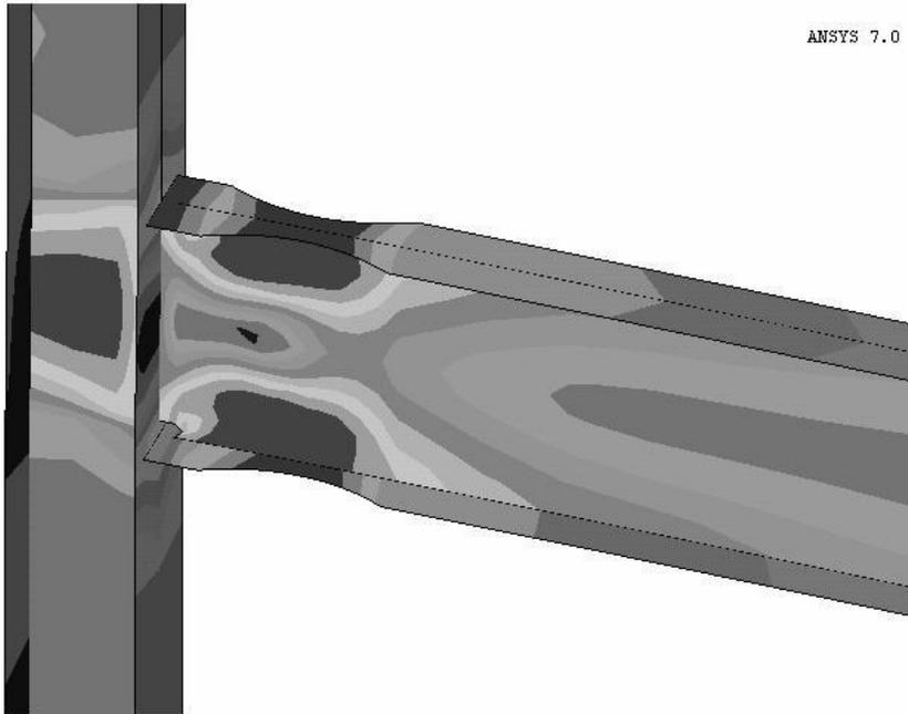
**Fig. 12: Oblique deformed view of the von Mises stress distribution in the RBS1 (W14x283 column) specimen at 0.015 radians.**
