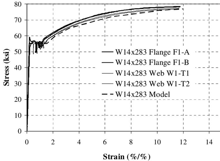
**Fig. 5: Stress versus strain curves for the W14x238 column.**
