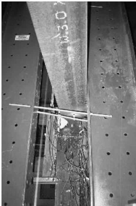
**Fig. 3: Observed lateral torsional buckling looking below the test specimen.**
