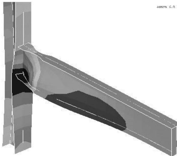
**Fig. 9: Isometric view of the RBS1 (W14x283 column) elastic buckling mode shape.**
