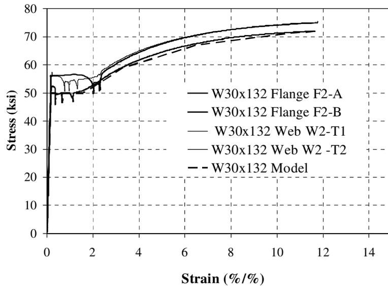
**Fig. 7: Stress versus strain curves for the W30x132 beam.**
