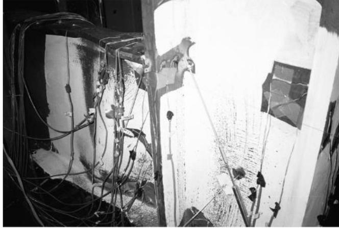
**Fig. 4: Localized beam web buckling and beam bottom flange deformation.**
