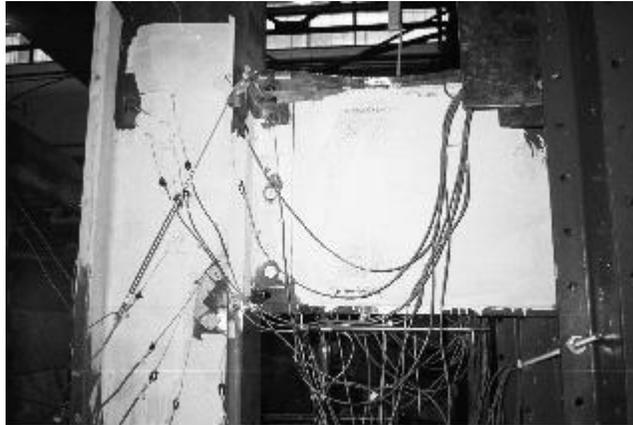
**Fig. 1: RBS moment connection specimen test set-up.**
