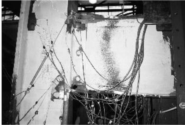
**Fig. 2: Observed whitewash flaking in the RBS and column panel zone.**
