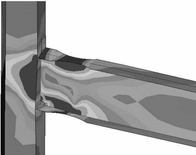
**Fig. 13: Oblique deformed view of the von Mises stress distribution in the RBS3 (W18x211 column) specimen at 0.015 radians.**
