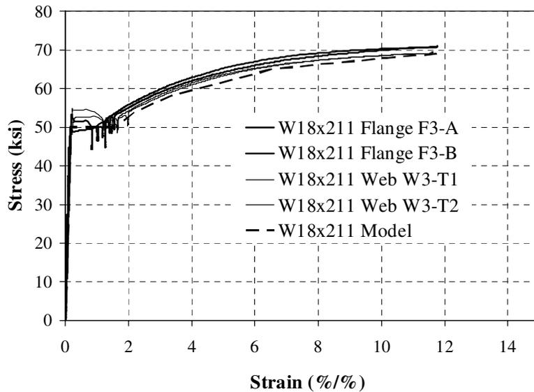
**Fig. 6: Stress versus strain curves for the W18x211 column.**
