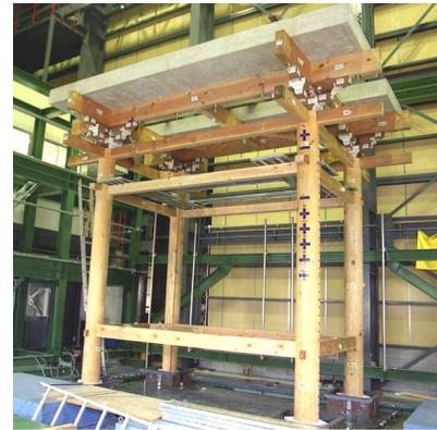
**Fig. 3 Full-scale model in shaking table tests**
