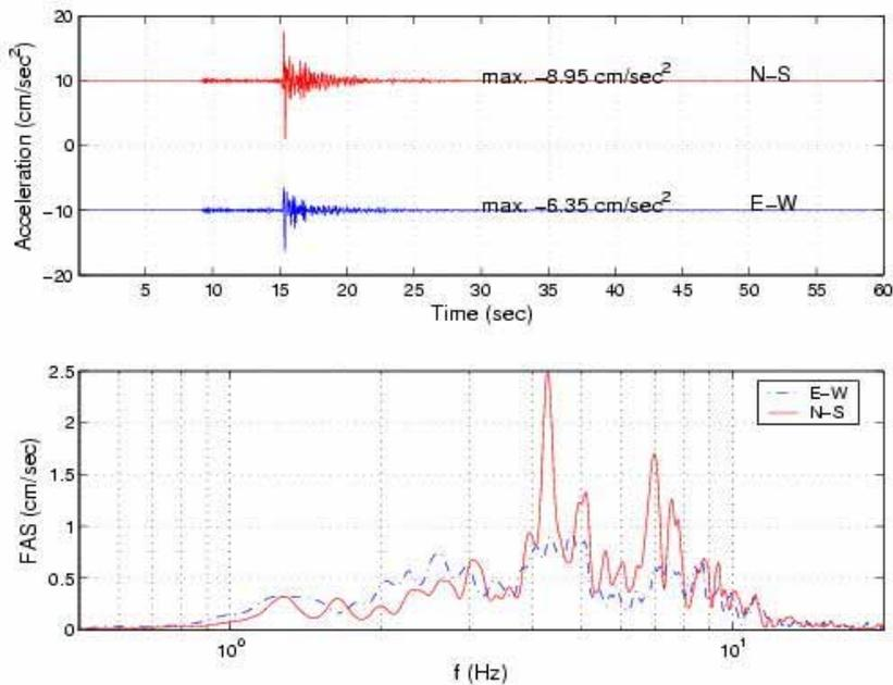
**Figure 5. Acceleration time histories and FAS of the input motions for the December 15, 2003 earthquake.**
