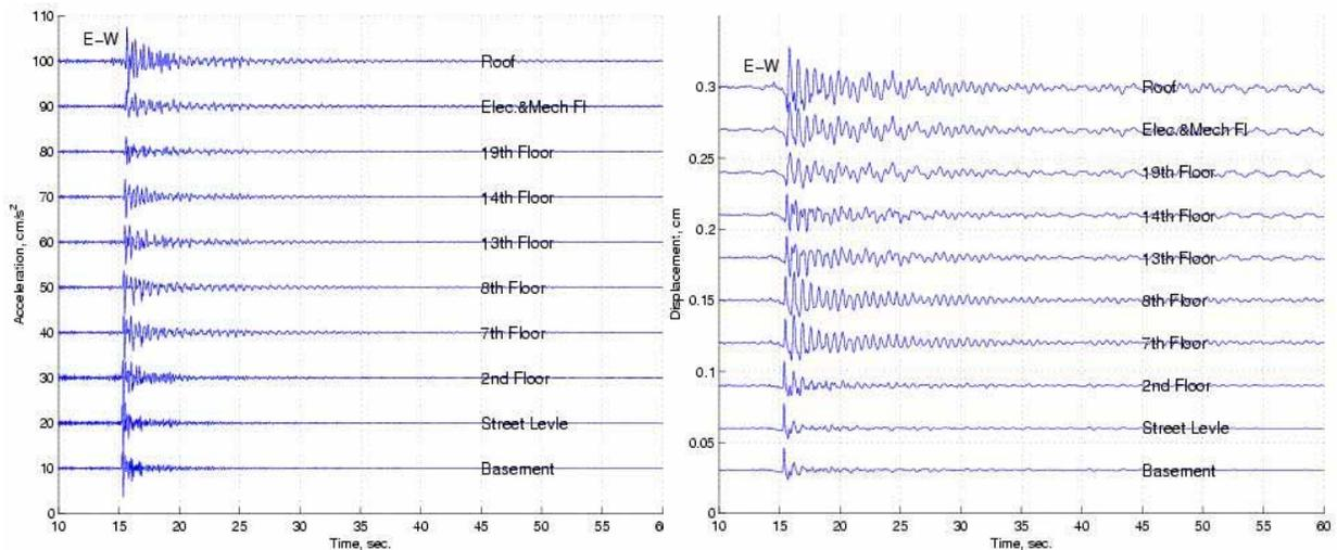
**Figure 6. E-W components of acceleration and displacement time histories for the December 15, 2003 earthquake.**
