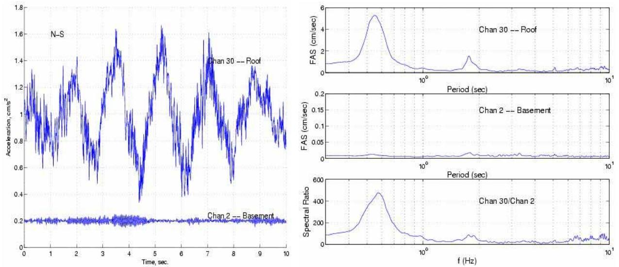
**Figure 11. Portion of N-W ambient test signals and their FAS recorded in the basement and roof level of the Atwood Building.**
