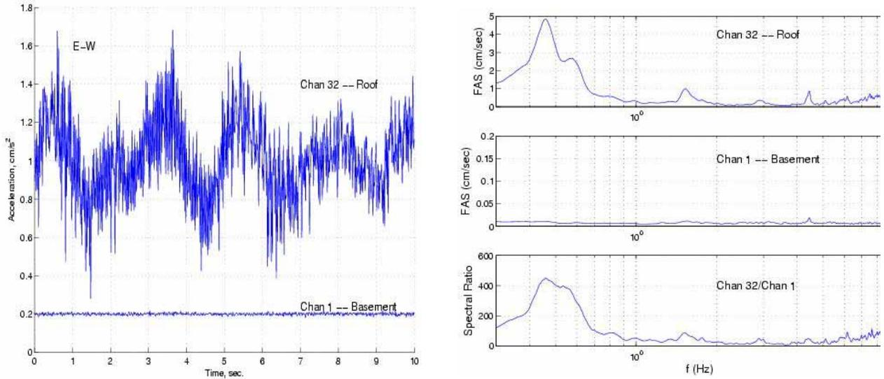
**Figure 10. Portion of E-W ambient test signals and their FAS recorded in the basement and roof level of the Atwood Building.**
