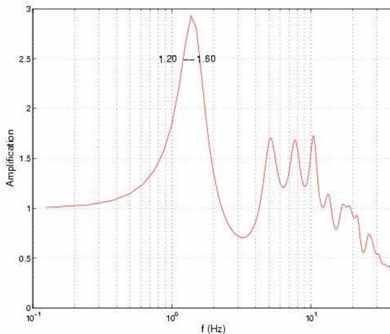
**Figure 13. Transfer function at the building site.**
