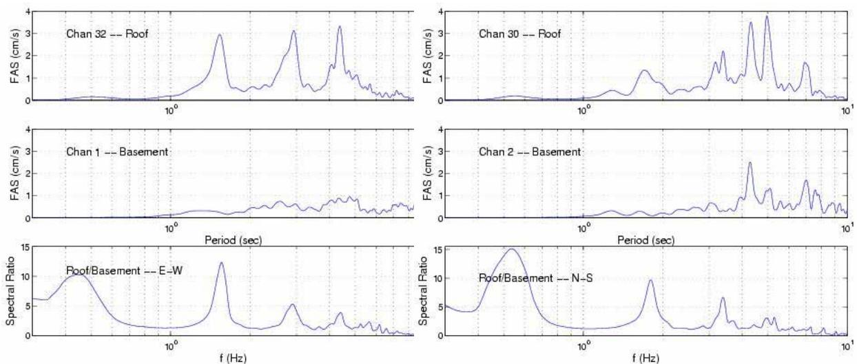
**Figure 8. Fourier spectra and spectral ratios based on recordings from the December 15, 2003 earthquake.**
