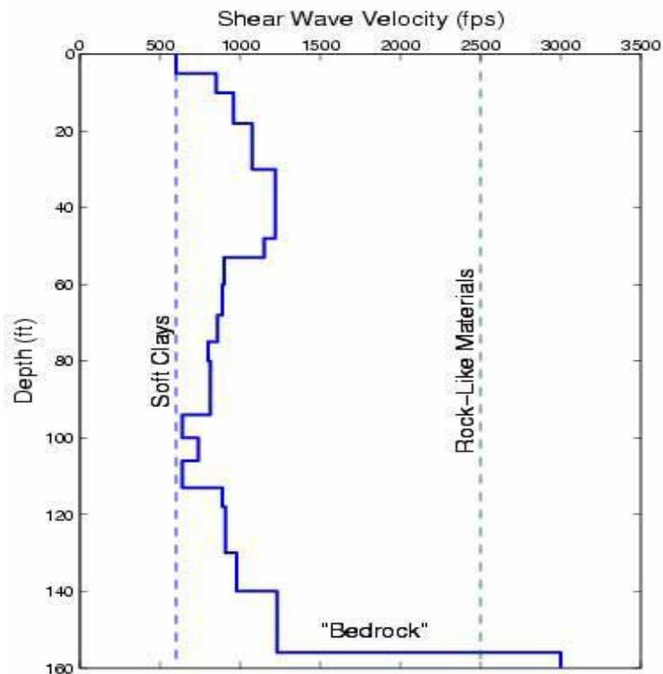
Figure 3. Shear wave velocity profile at the Atwood Building site.
