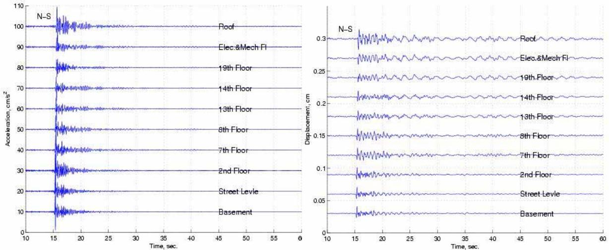
**Figure 7. N-S components of acceleration and displacement time histories for the December 15, 2003 earthquake.**
