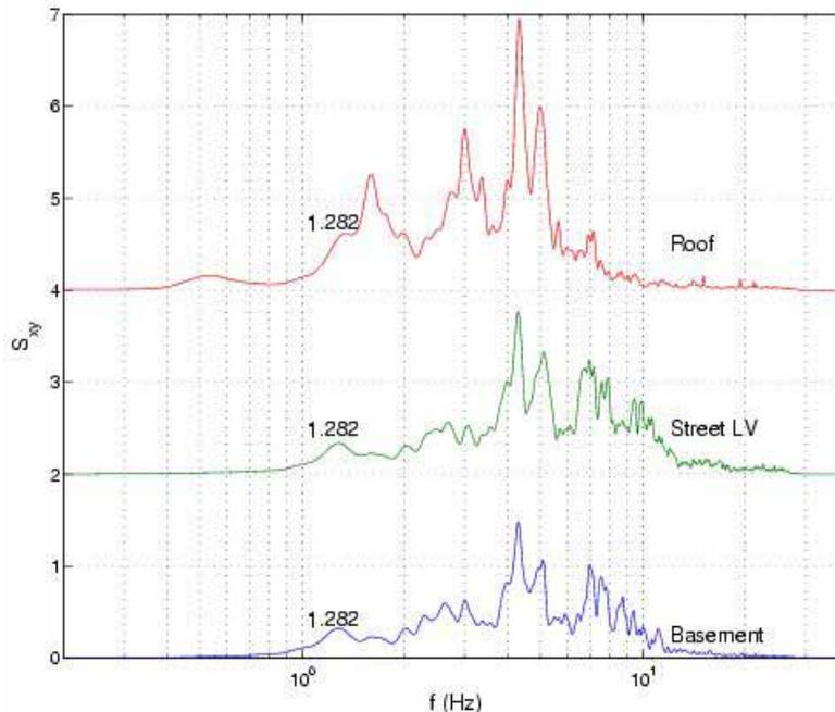
**Figure 12. Cross-Spectra of motions at the roof, street level and basement of the Atwood Building.**
