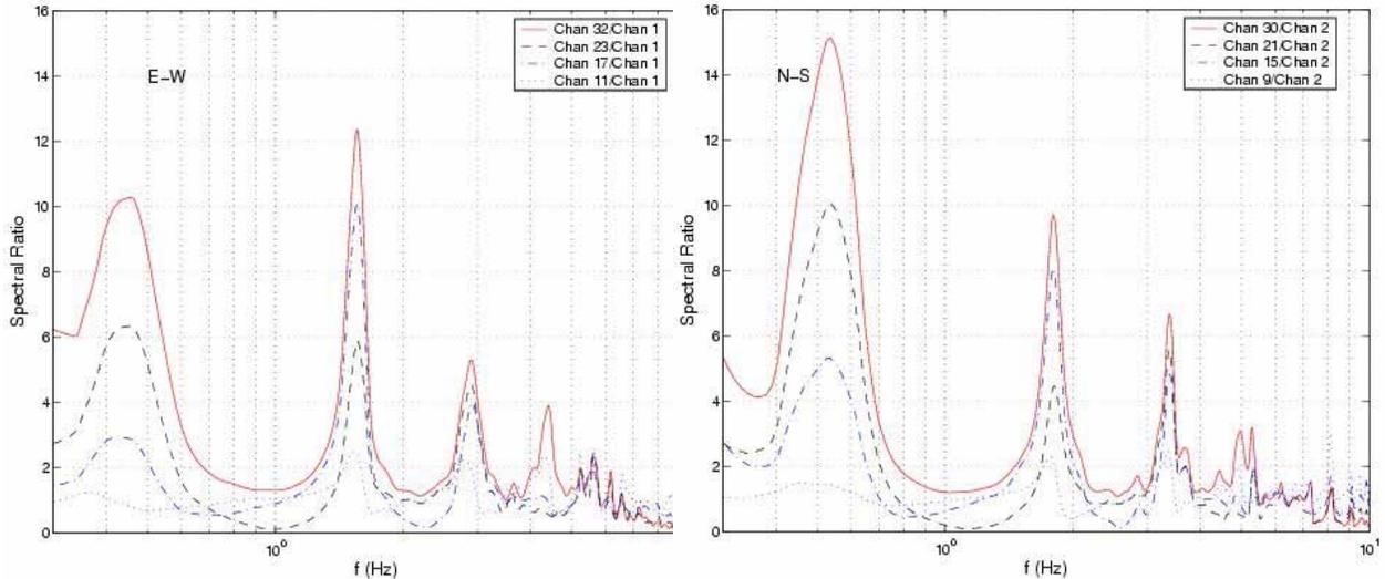
**Figure 9. Spectral ratios computed at four different building levels using the December 15, 2003 earthquake data.**
