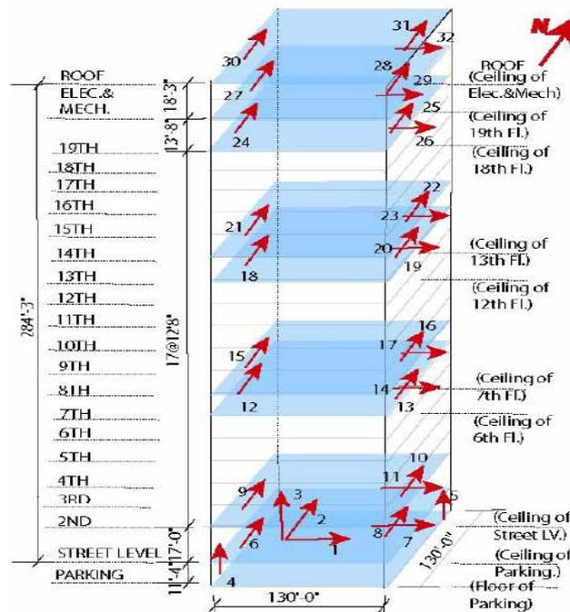
Figure 4. The seismic sensor configuration in the Atwood Building.
