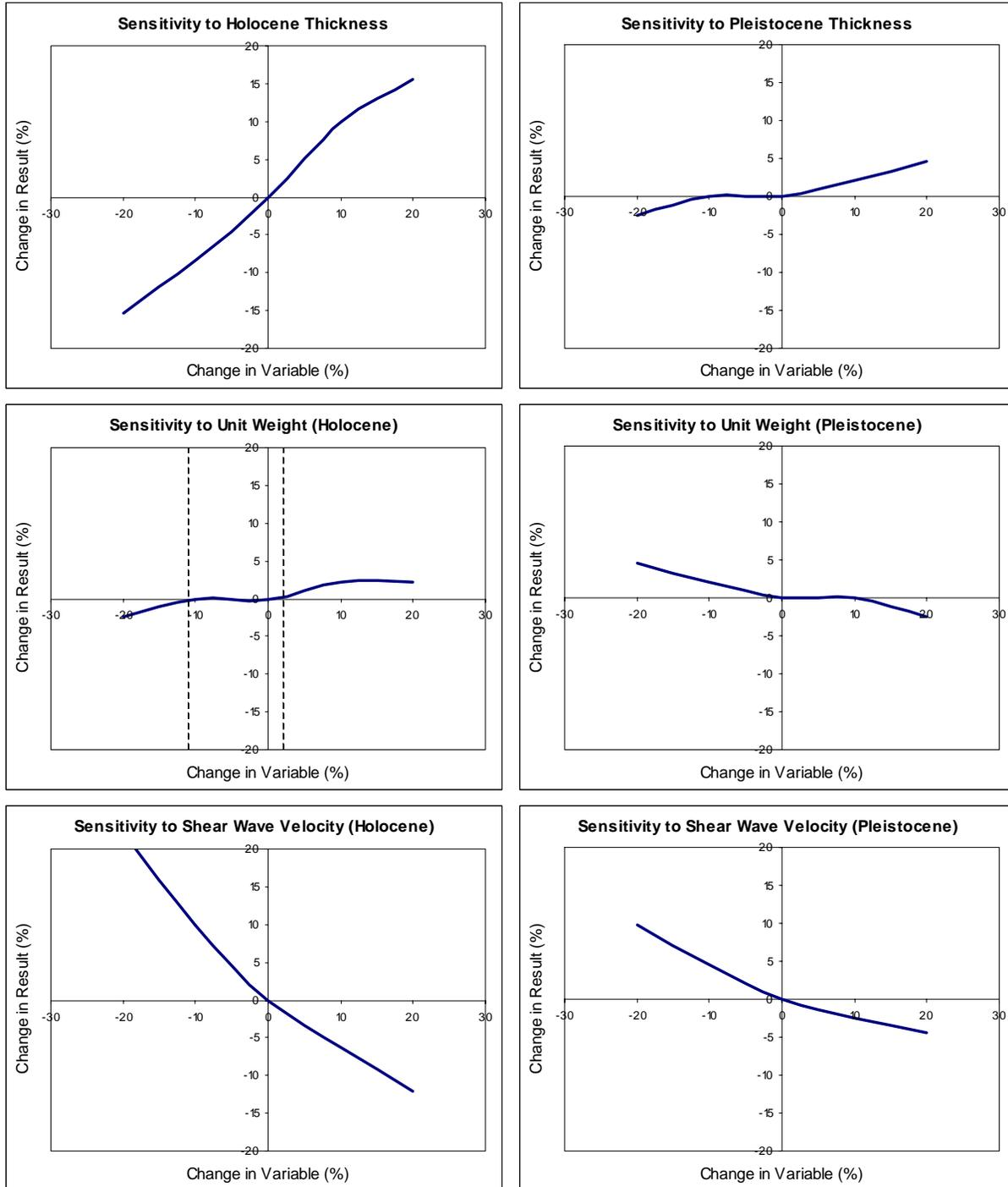
**Figure 10. Sensitivity of site periods to soil properties**
