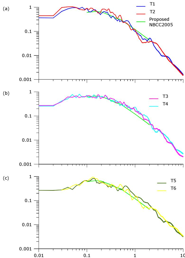
**Figure 2– Uniform Hazard Spectra for a selected Eastern Canada site, according to the proposed 2005 edition of the National Building Code of Canada (Adams *et al* [13]), compared with spectra for records (a) T1, T2; (b) T3, T4; and (c) T5, T6.**
