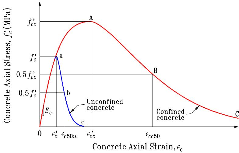
**Figure 1 - Stress-strain relationship of confined concrete - Légeron and Paultre [10]**
