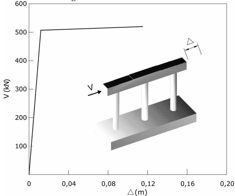
Figure 5 - Pushover and bridge bent for bridge S1
