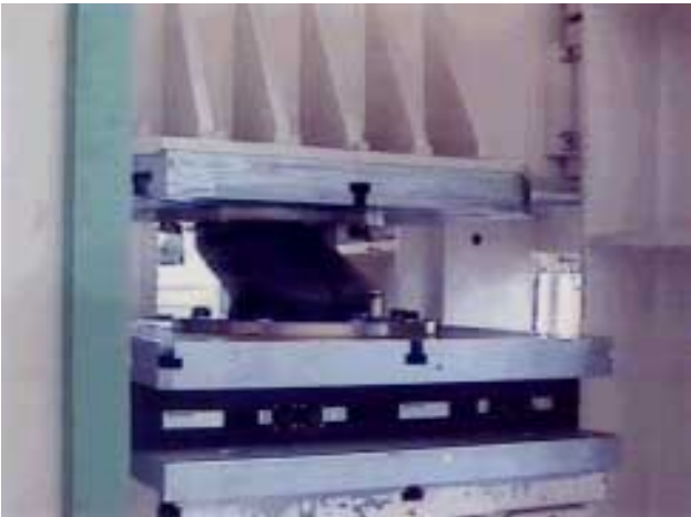
Figure 22 Static test of flat shape rubber bearing
