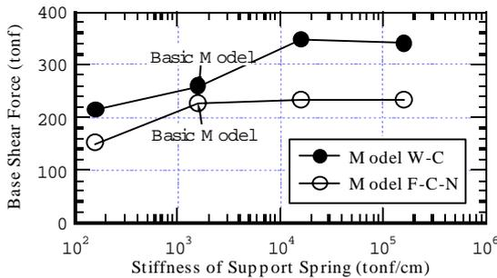
**Figure 15: Effect Of Support Stiffness**
