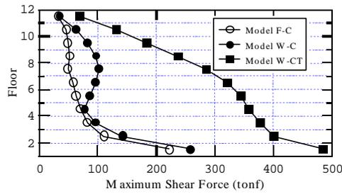
**Figure 12: Maximum story shearing force of inter story**
