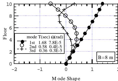
Figure 5: Aspect Ratio and Natural Period Figure 6: Mode Shape and Rotation Angle at Base
