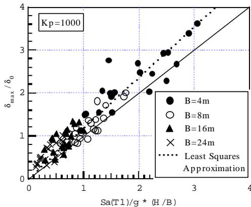
**Figure 7: Uplift Displacement and Acceleration Response Spectrum**
