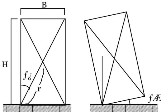
Figure 1: Motion of Rigid Body
