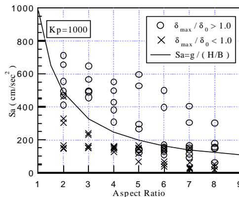
**Figure 8: Presumption of Uplift Condition**
