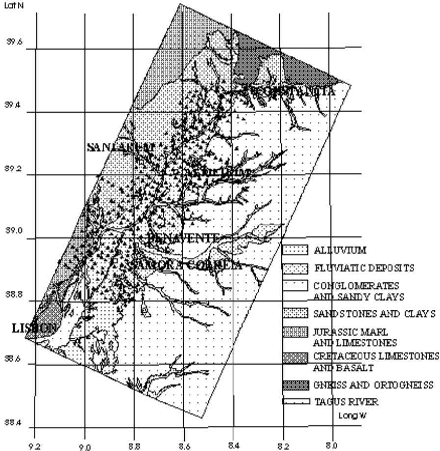
Figure 2 – Sketch of the geological map of the Lower Tagus Valley region (adapted from SPG, 1992). The small triangles indicate the recording sites of the large scale microtremor survey.
