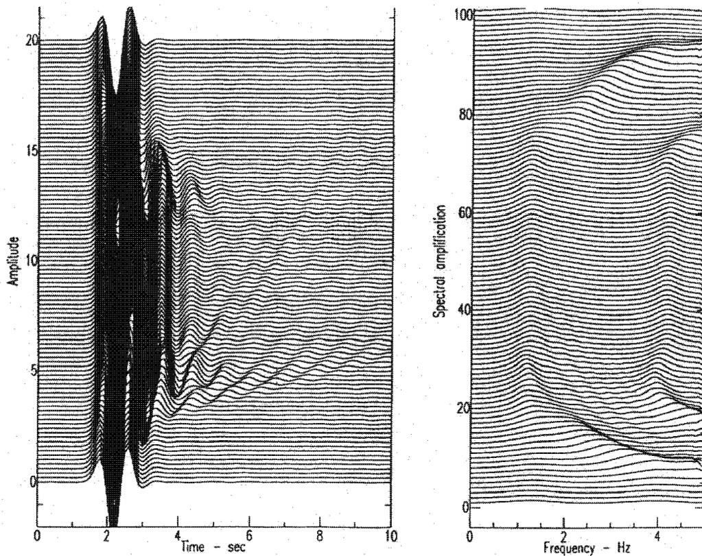
**Figure 7 – 2D response obtained in 100 points equally spaced along the cross-section of the valley. (a) On the left: synthetic seismograms; (b) on the right: spectral amplification.**
