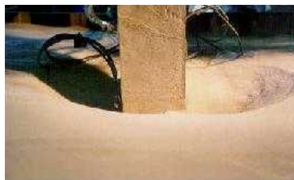
Figure 7 : Photo of Ground Surface around Pile
