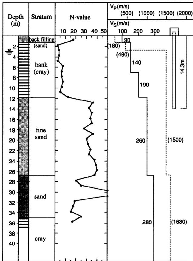
Fig. 2. Soil profile in test yard.
