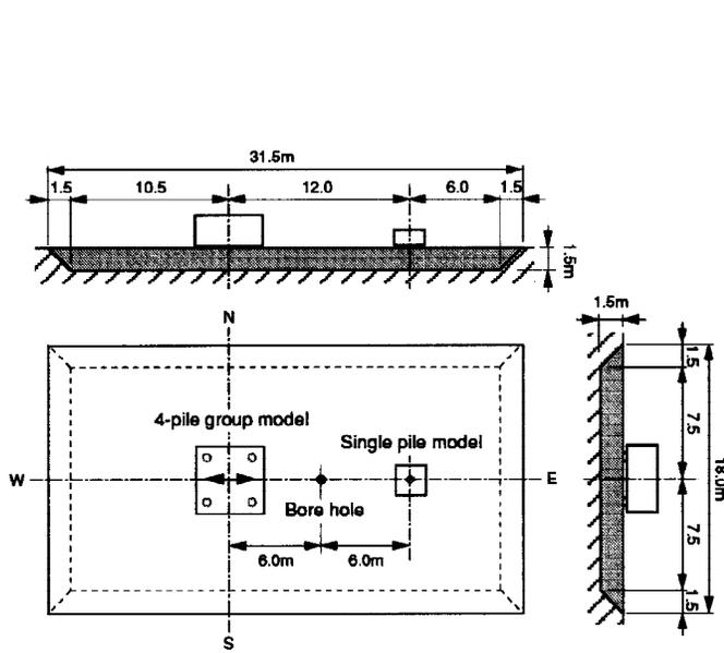
Fig. 1. Test yard and layout of test models.
