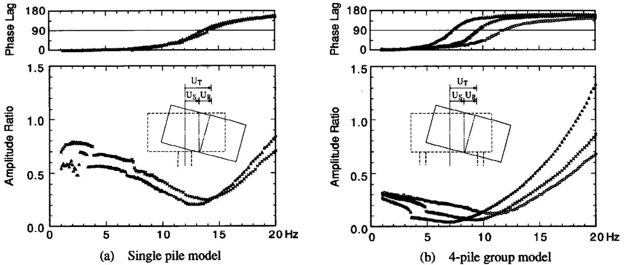
Fig. 6. Amplitude ratio and phase lag of rocking displacement against swaying one,  $U_R/U_S$ .
