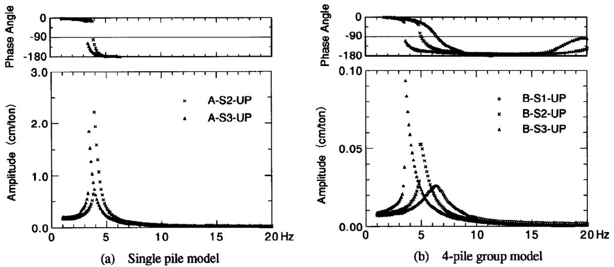
Fig. 4. Resonance curves of horizontal displacement at top of block,  $U_T$
