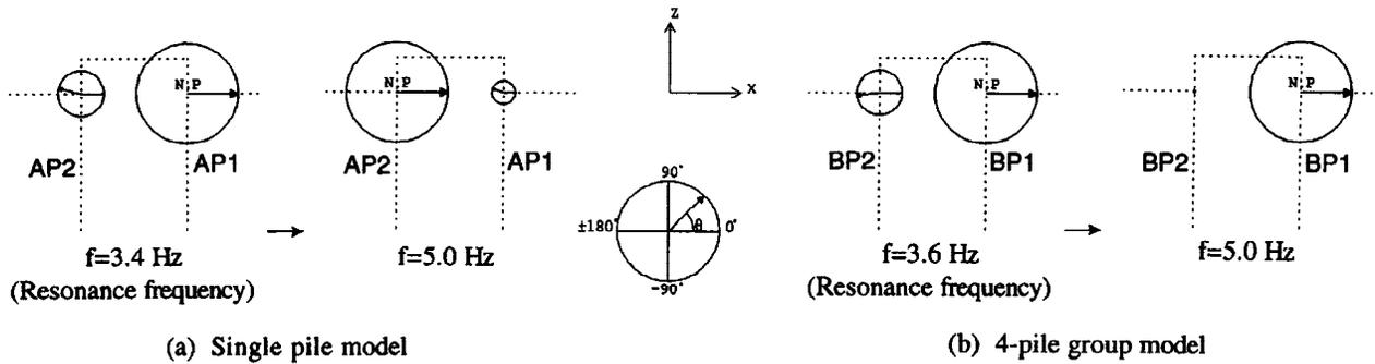
Fig. 5. Distribution of earth pressure at resonance frequencies in the case of S3-UP.
