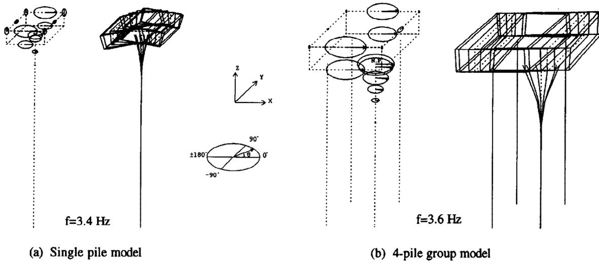
Fig. 7. Mode shapes of vibration at resonance frequencies in the case of S3-UP.
