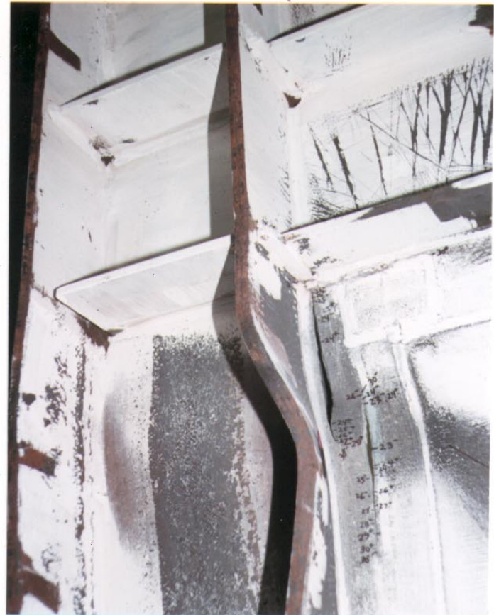
Figure 4: Tearing of shear plate at corner locations
