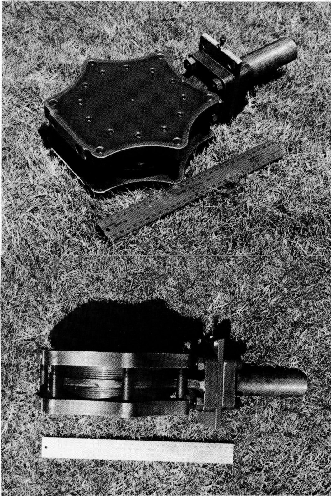
Figure 1. The self contained Lead-Shear Damper. Shown is a 200 kN damper with a stroke range of \pm 2 micro metres to \pm 10 mm.
