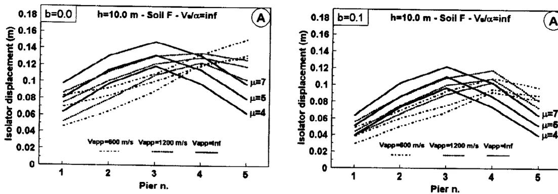
Fig. 3b) - Bridges  $H = 10,0$  m. Total hardening = 0,0 and 0,1. Isolators displacement for  $v_s/\alpha = \infty$  m/s.
