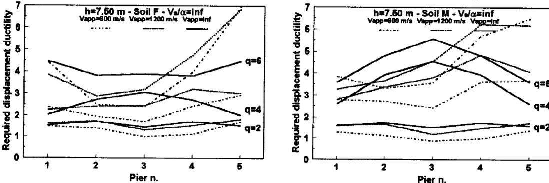
Fig. 2b) - Conventional bridges  $H = 7,5$  m on soil F and M. Required ductility for  $v_s/\alpha = \infty$  m/s.
