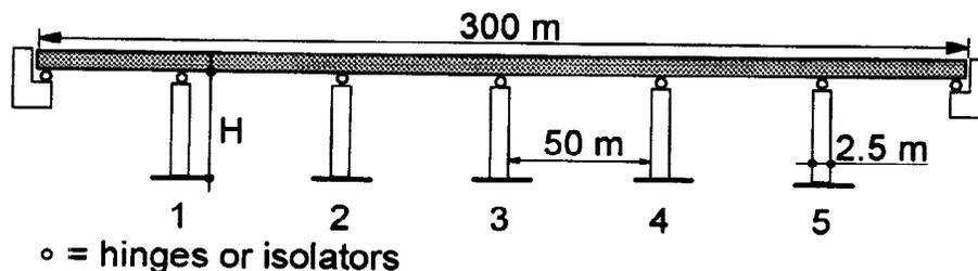
Fig. 1 - Schematic geometry of the analyzed bridge
