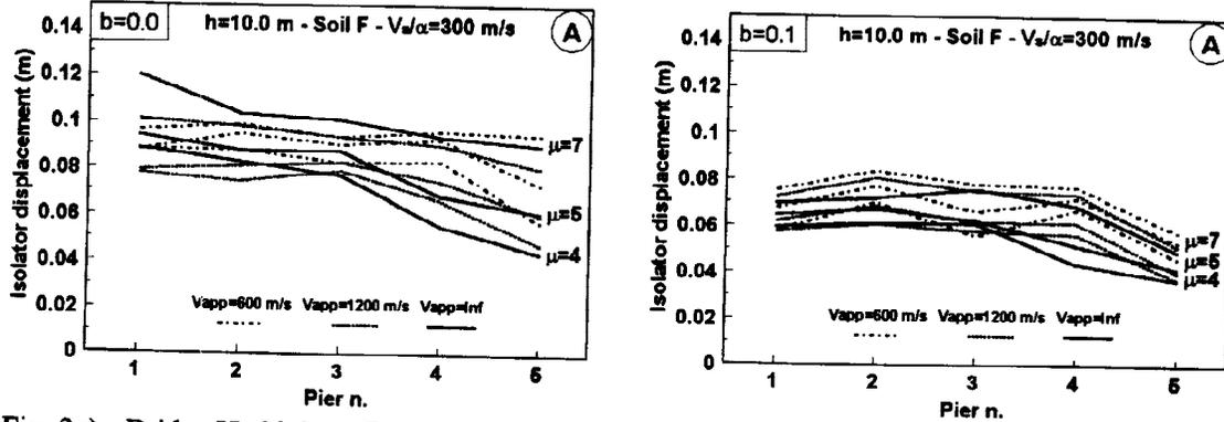
Fig. 3a) - Bridge  $H=10.0$  m. Total hardening = 0.0 and 0.1. Isolators displacement for  $v_s/\alpha = 300$  m/s.
