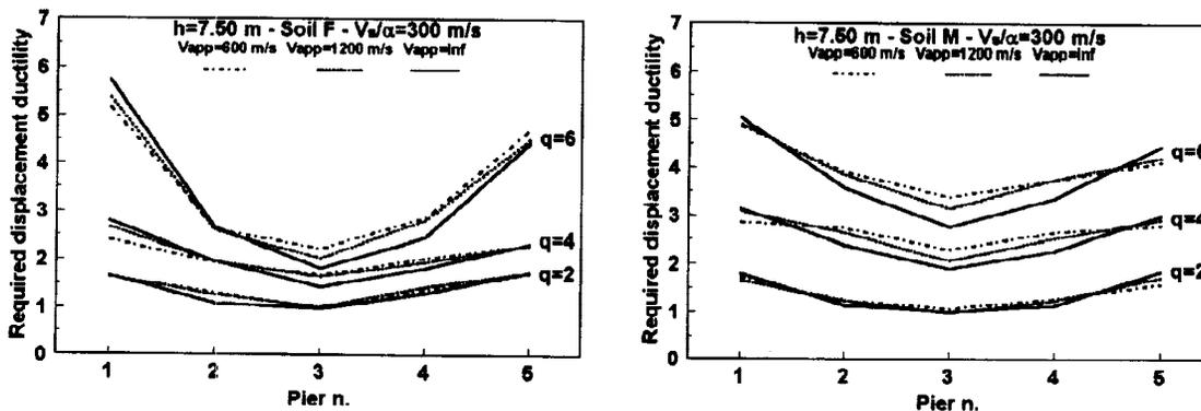
Fig. 2a) - Conventional bridge  $H=7.5$  m on soil F and M. Required ductility for  $v_s/\alpha = 300$  m/s.
