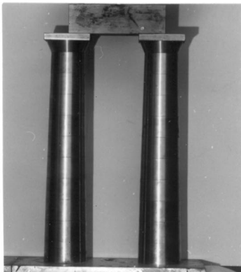
Figure 15. System on the Shaking Table
