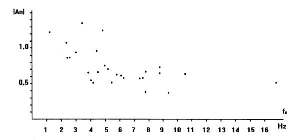
Fig. 1. The diagram of spread in maximum values of Fourier coefficients of accelerograms for prevailing frequences
