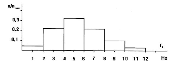
Fig. 2. The bar chart of accelerograms prevaling frequences
