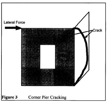
small compared to the strength of the spandrels, a flexural crack will occur at the top of the pier. Since the pier is unreinforced, the maximum shear force that can be transferred to the pier will have been reached and
