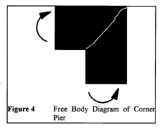
corner of the wall. Third, at the top of the building, there is little dead load on the pier that needs to be overcome to produce a net tension - and thus cracking - due to the moment. These factors produce a condition where the rocking block cannot occur. A free body diagram at the unreinforced joint at the top corner demonstrates that a diagonal crack will develop, as shown if Fig. 4.
