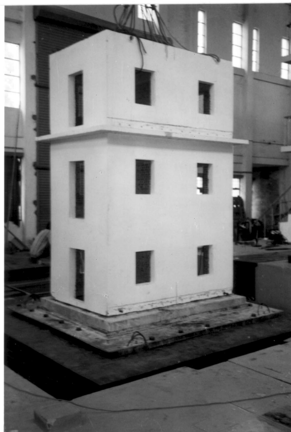
Fig. 1. Test structure: a) Configuration, and b) Structure on shaking-table during the experiment.
