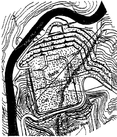
Fig.1. The plane view of the created land and the contour line of original ground surface.
