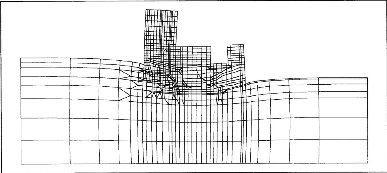
Fig.2a Strained Structure - loads:weight
