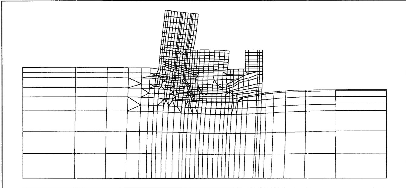
Fig.2b Strained Structure - loads : weight + water pressure
