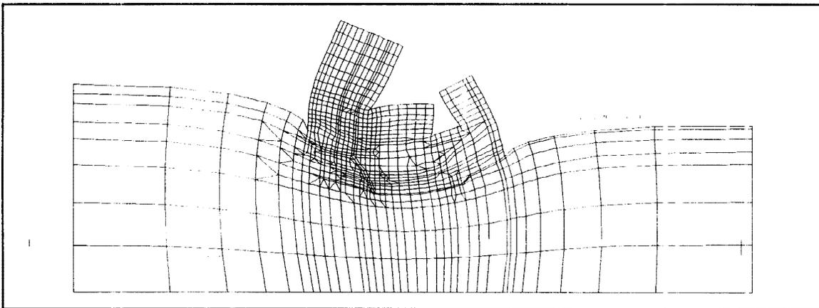
Fig.3b Frequencies and Mode Shapes no.2
