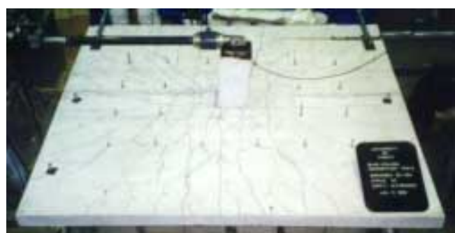
Figure 10: Specimen 4HS at 8% drift.
