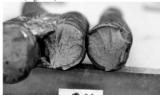
Figure 7: Fracture surface of lap joint sample MMAW 500E - 32 mm bar
