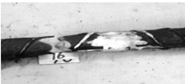
Figure 4: Grade 300E 32mm bar following tensile test bar
