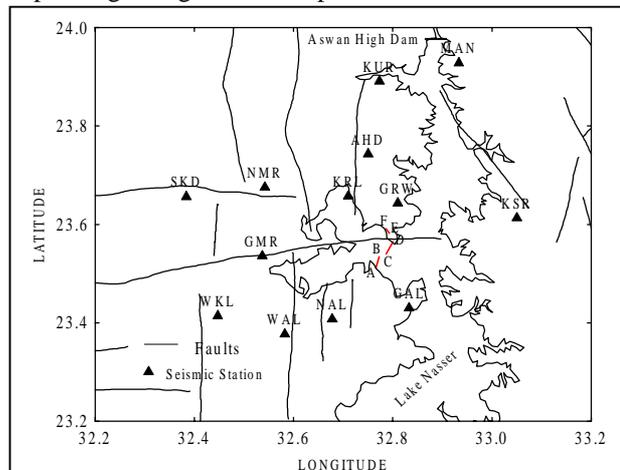
**Fig. (1) Proposed Kalabsha Dam as represented by three segments AB, CD, and EF (solid Lines denote the faults around the dam and solid triangles represent the telemetry seismic stations)**
