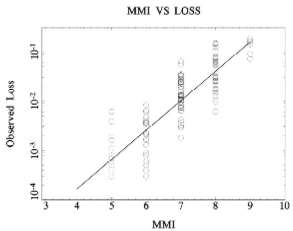
**Figure 2** Observed loss vs. MMI, Northridge earthquake
