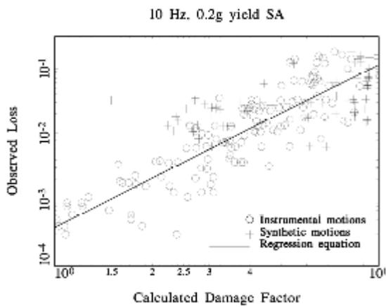
**Figure 3** Observed loss vs. Damage Factor DF
