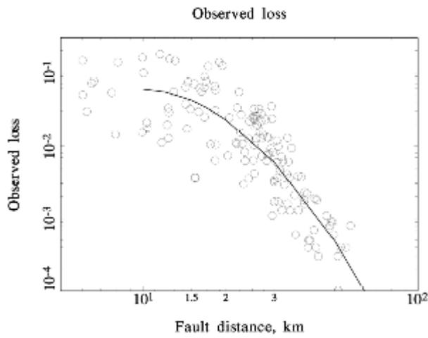
**Figure 1** Observed loss vs. distance, Northridge earthquake
