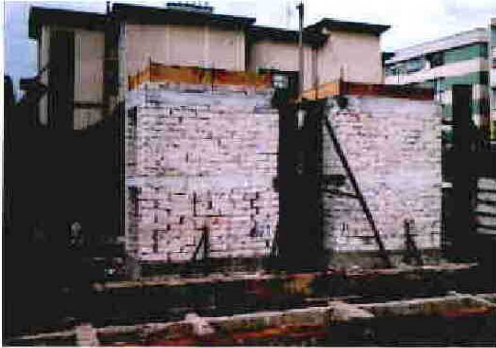
Fig. 6. Masonry models tested on a shaking table. (Olaru)
