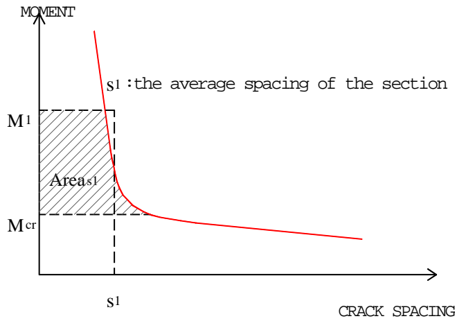
Figure 2 Relationship between Moment and crack spacing
