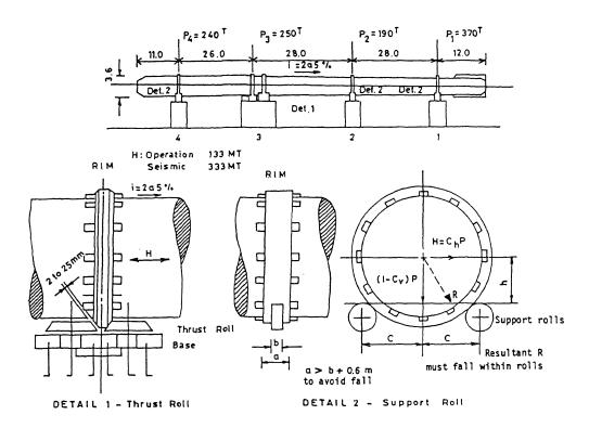
In this case, because of the large heat expansions, all the longitudinal seismic force must be resisted at support  $N^{\circ}$  3. Special thrust rolls, with a capacity 2.5 times the standard in non seismic areas were required. If this fact is not detected at the early stages of the quotations and purchase negotiations it is almost certain that delays, claim and loss of good will will follow.
