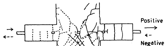
Fig. 4 Crack patterns observed at No.5 specimen which failed in bond
