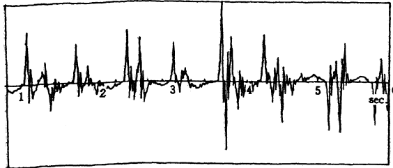
Fig. 10 Bending moment M developed at the tank wall (Max. value 0.13 \text{ N}\cdot\text{cm}/\text{cm} )
