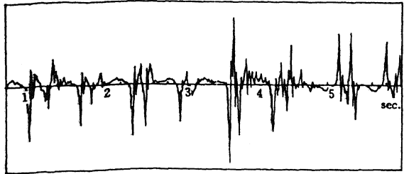
Fig. 9 Axial force N , developed at the tank wall (Max. value 571 \text{ N}\cdot\text{cm}/\text{cm} )
