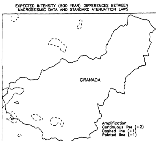
Figure 6: Differences between our revised and new set of single points and Martín Martín (1984) attenuation law results for expected intensities during the next 500 years.
