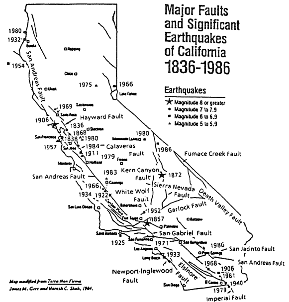
Figure 2. Faults and significant historical earthquakes of California (Bertero, 1991)
