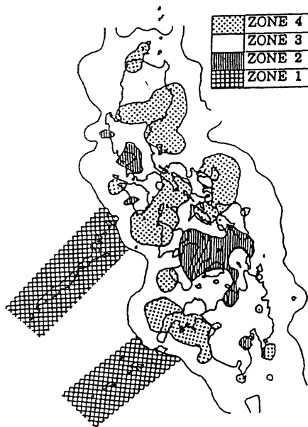
Figure 10. Proposed seismic zoning map for the Philippines based on the expected peak ground acceleration.
