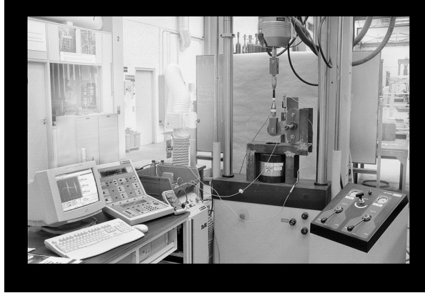
Figure 3: Setup of the damper tests with Instron machine
